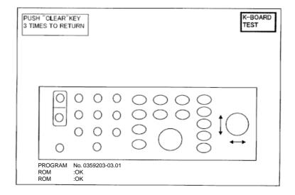
Screen for testing keyboard, remote controller
